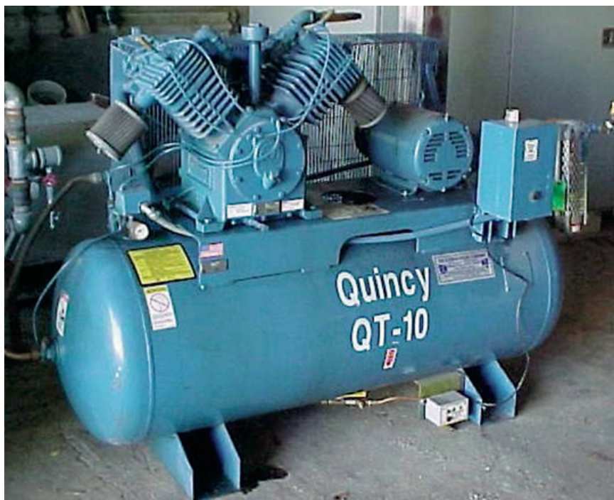
A compressor will generally use its purchase price in electricity every year, so selecting and efficiently operating the correct type of compressor for the application is essential.
