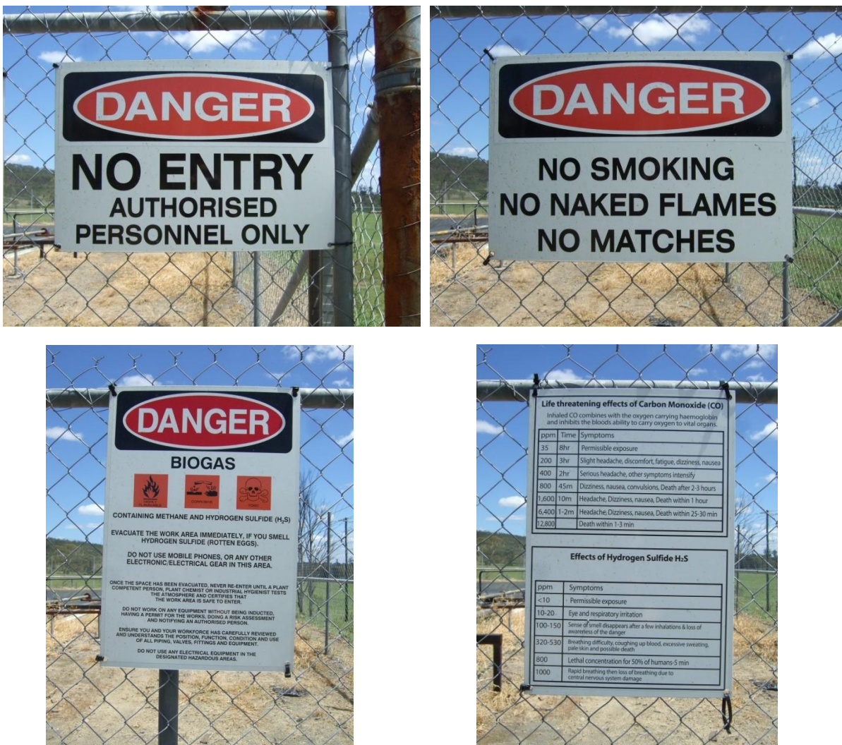
Image 8: Suitable safety signs on exclusion zone
