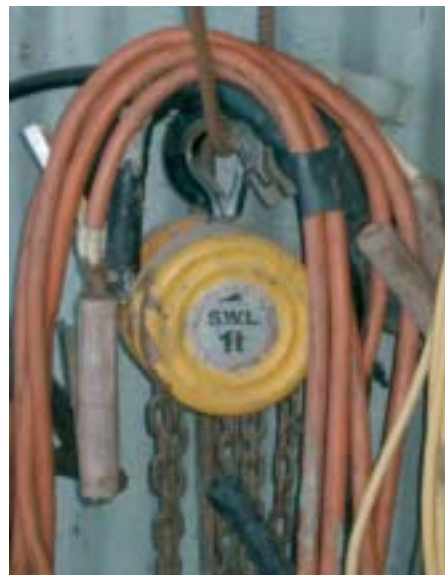
Clearly visible safe working limit
