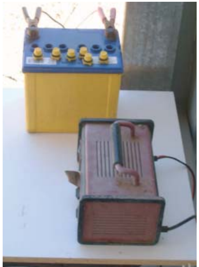
Right: Battery charging in a well ventilated area
