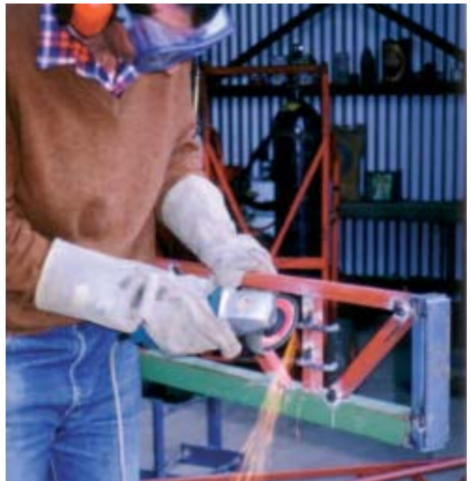
Operation of angle grinder using appropriate protective equipment
