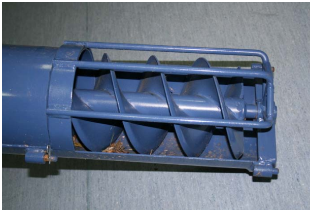
Lugs welded to the inner guard to attach the outer guard
