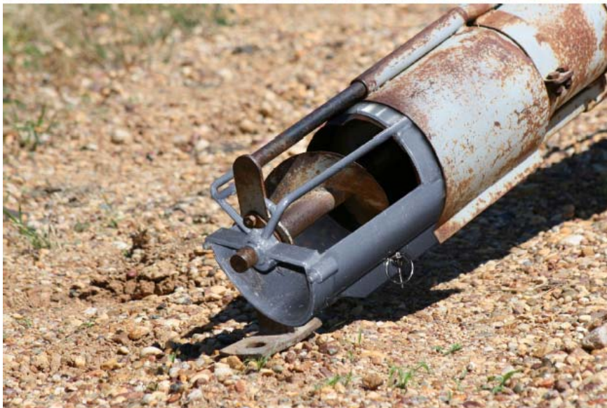
Old auger with inner guard retrofitted
