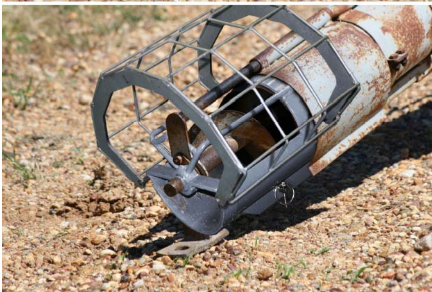
Old auger with both inner and outer guards retrofitted
