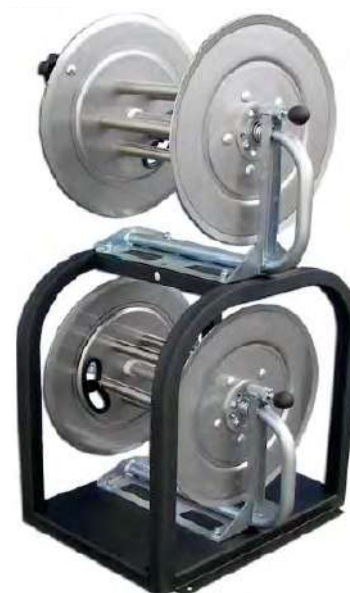
SAVE SPACE ... HAR325 2 reels, double stacked, one HAR151 + one low pressure supply reel with capacity for 45m low pressure hose
