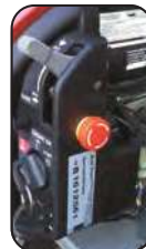
Emergency stop fitted
