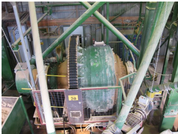
Plate 1: Ball mill used to reduce crushed rock to powder (photo source: Gordon Heath, 2009).
