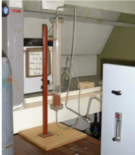
Figure 13. Photograph of the column used for testing on site and in the laboratory.
