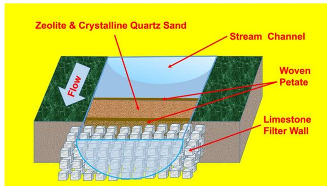
**Figure 4.** Hypothetical scheme of the ancient water purification system at Tikal. Macro-crystalline quartz crystal sand and zeolite filtration system positioned just upstream of, or within the reservoir ingress. Kenneth Barnett Tankersley used Microsoft PowerPoint for Mac Version 16.41 ([www.microsoft.com](http://www.microsoft.com)) to create this figure.
