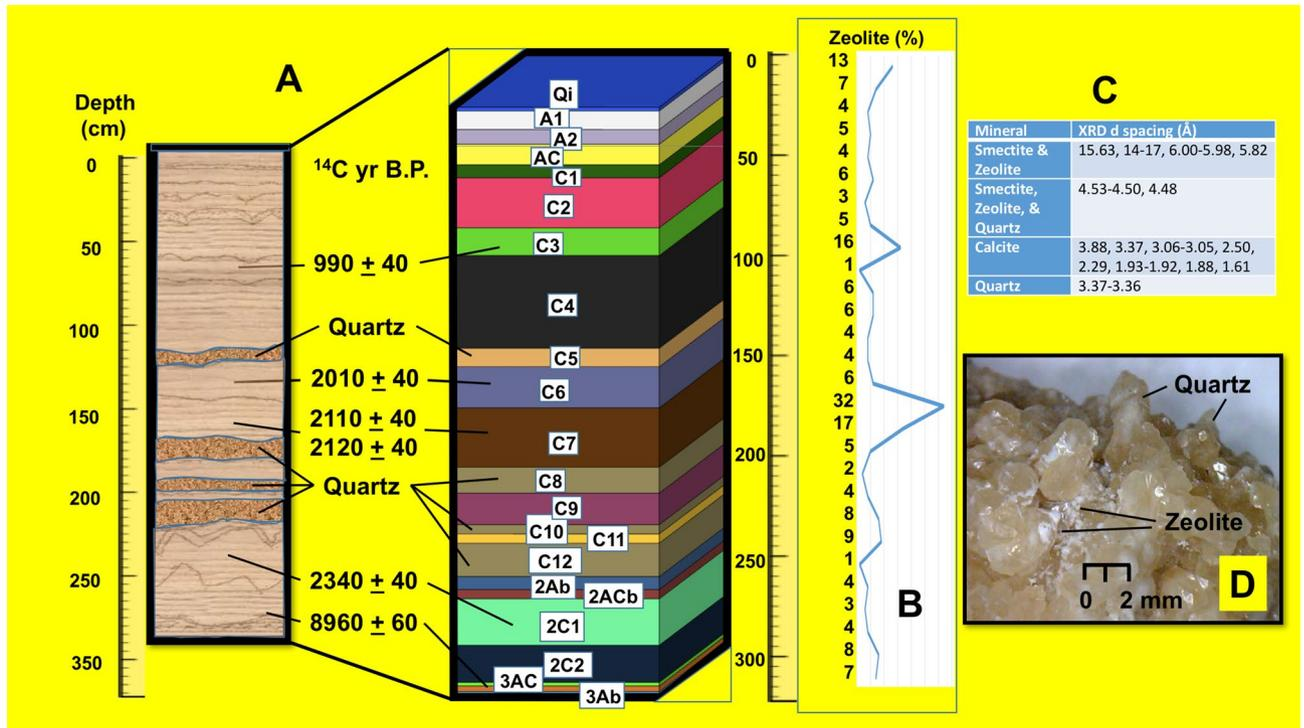
**Figure 3.** Chronostratigraphy of the Corriental reservoir. (A) Soil horizons and sediments of the Corriental reservoir showing the location of anthropogenic quartz and radiocarbon ages yr B.P. (B) Relative percent of zeolite by depth. (C) Distinctive mineral XRD peaks. (D) Photomicrograph of anthropogenic euhedral quartz crystals and zeolite. Kenneth Barnett Tankersley used Microsoft PowerPoint for Mac Version 16.41 ([www.microsoft.com](http://www.microsoft.com)) to create this figure.
