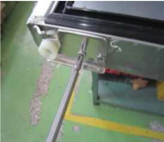
F. Disassemble stopper plate, then tight screws.
