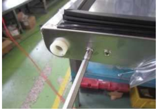
G. Assemble stopper plate in original positions.
