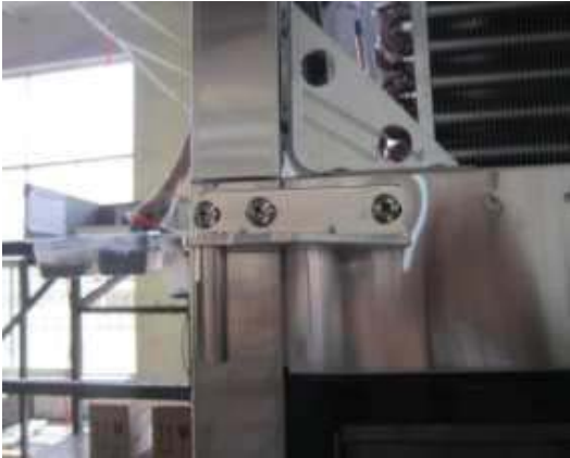
F. Disassemble stopper plate, then tight screws.
