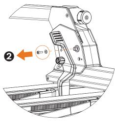
Using the 6mm Hex Key, remove the four M10 countersunk screws connecting the Lower End to the centerbeam. The Lower End can now be removed.
