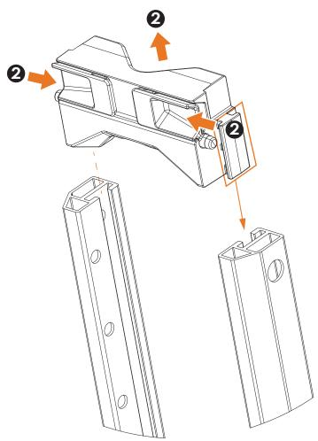
(3) Install the new Tire Chock and reassemble the tire arm bridge by following steps 1 & 2 in reverse. Torque the two M6 screws to 12 Nm.
