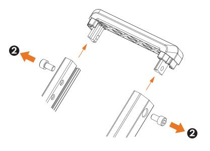
Remove Tire Arm Chock from Tire Arm T-channels.
