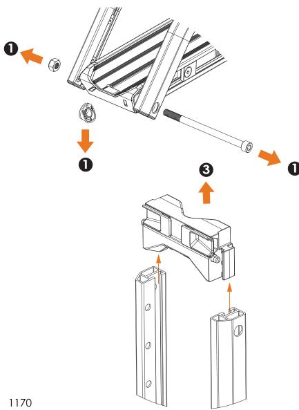
Remove Tire Arm Bridge from Tire Arms with M6 bolts and Tire Arm Bridge Mounting Nuts attached.
