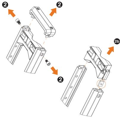
4 Install the new Tire Arm and reinsert the Tire Arm Bridge and hardware by following steps 1, 2 & 3 in reverse. Torque the Tire Arm Linkage Bolt to 20 Nm., torque the two M6 screws to 12 Nm and torque the Tire Arm Pivot Bolt to 16 Nm.
