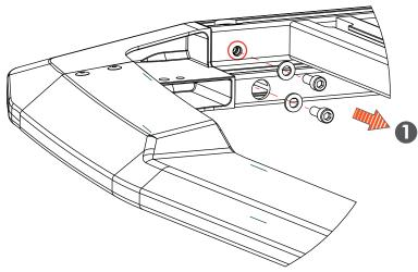
3 Install two new M6 square nuts into each corner of the new Nose.
