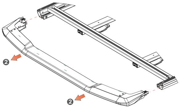
2 Remove the Nose and Tail from the rack.
