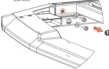
3 Using the 4mm Hex Key, remove the M6 countersink screws from the crossbars. Retain the countersinks, spacers, and t-nuts. Remove the Side Extrusion.
