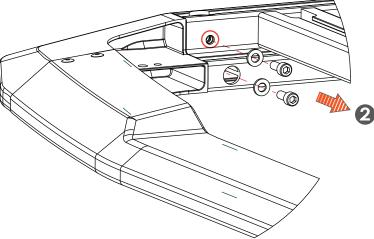
Using the 4mm Hex Key, remove the M6 countersink screws from the crossbars. Retain the countersinks, spacers, and t-nuts. Remove the Side Extrusion.
