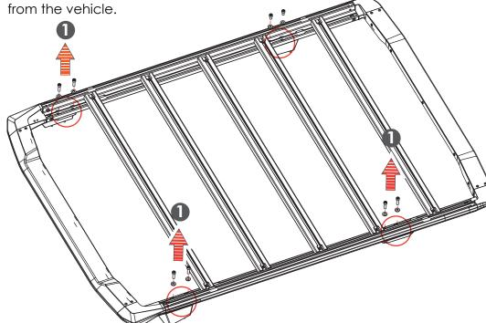
2 Using the 5mm Hex Key, remove the eight M6 bolts from the nose and tail corners.
