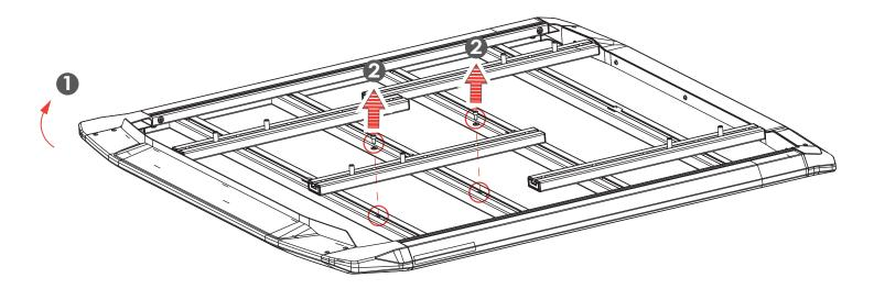
3 Replace the old crossbar T-Nuts with the provided new T-nuts.
