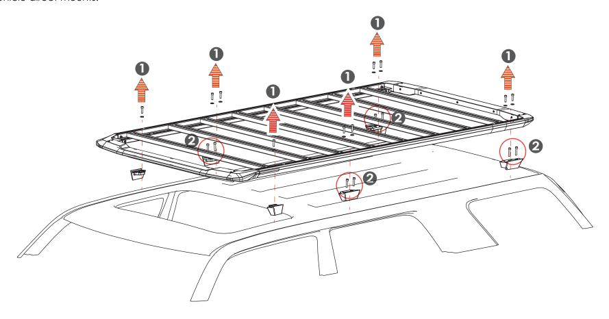
(3) Install the new Direct mounts. Take note of the Mount positions. Torque the M8 screws to 20 Nm.
