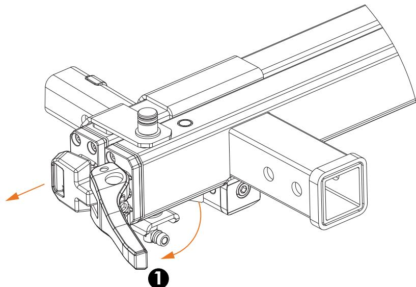
② Using the 5mm Hex Key, remove the seven M8 bolts. The Pivot Latch and Hook can now be removed.
