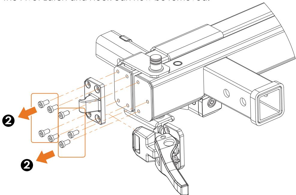
③ Install the new Pivot Latch and hook by following Step 2 in reverse. Torque the M8 bolts to 29 Nm.
