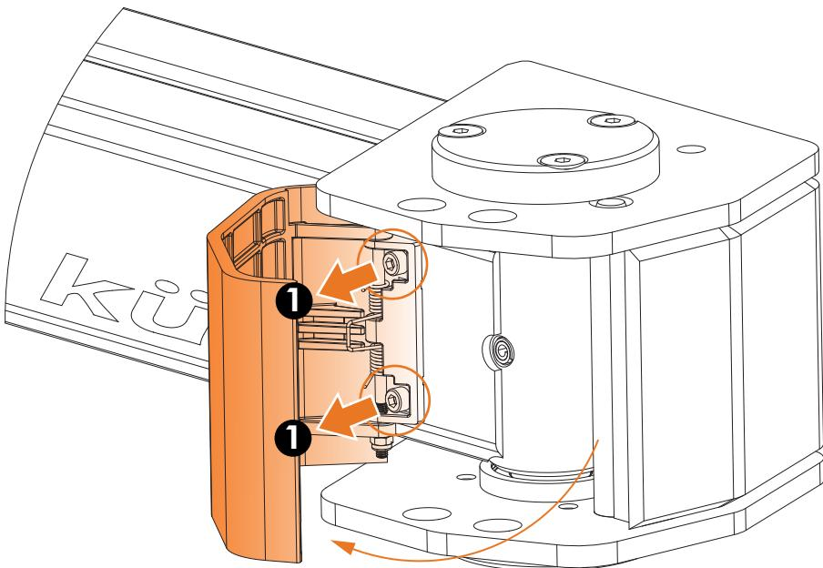
② Install the new Pivot Shroud; **do not remove** the cardboard installation tool until after the M6 Screws are threaded. Using the 4mm Hex Key, torque the M6 Screws to 9 Nm.
