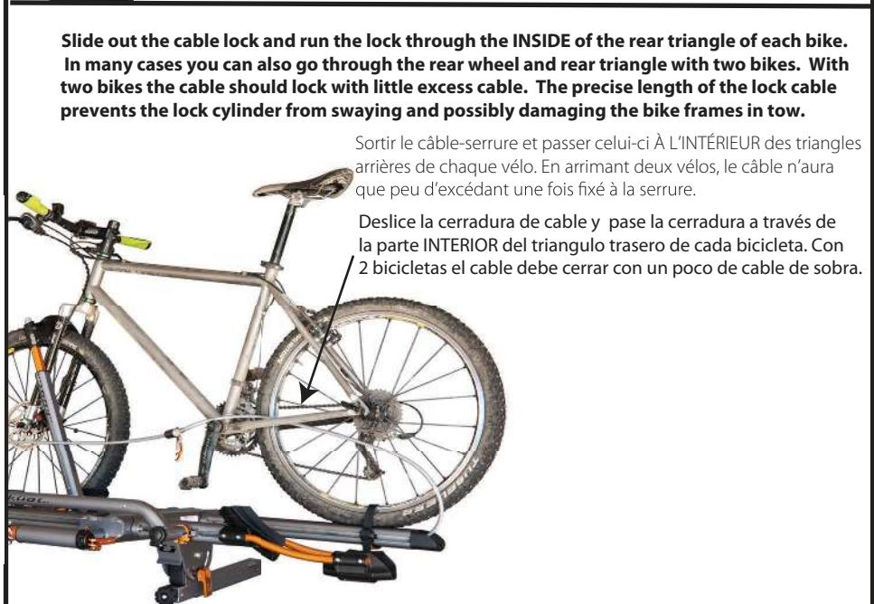
**Slide out the cable lock and run the lock through the INSIDE of the rear triangle of each bike. In many cases you can also go through the rear wheel and rear triangle with two bikes. With two bikes the cable should lock with little excess cable. The precise length of the lock cable prevents the lock cylinder from swaying and possibly damaging the bike frames in tow.**
