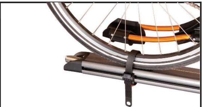
**Slide the rear tire strap through the center of the rear tire. Push the strap through the ratchet and pull tight.**
