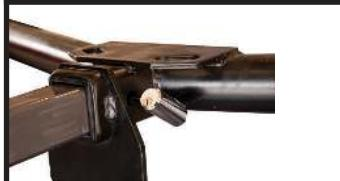
**Slide the locking hitch pin through the hitch and lock.**
