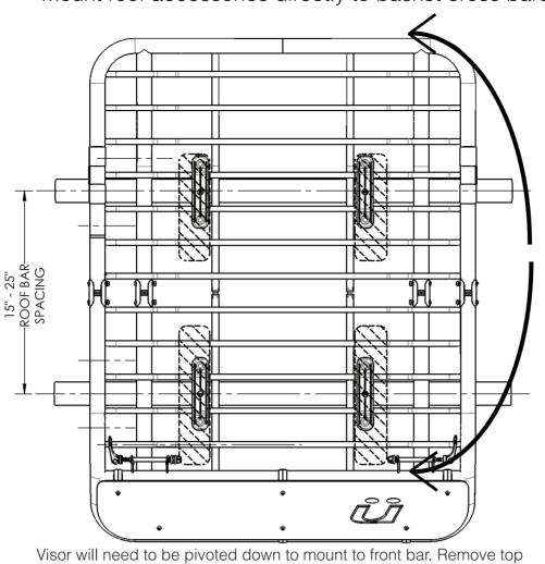
3 visor clamps to pivot. Visor will stay attached to basket.
