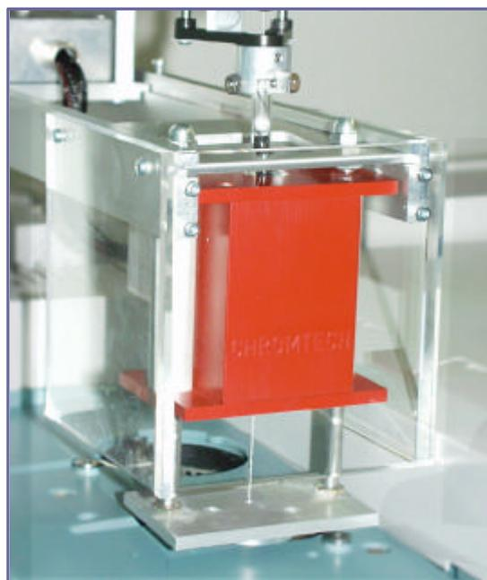
Fig. 2: TDAS 2000 desorption unit with GC 6890 and PTV.
