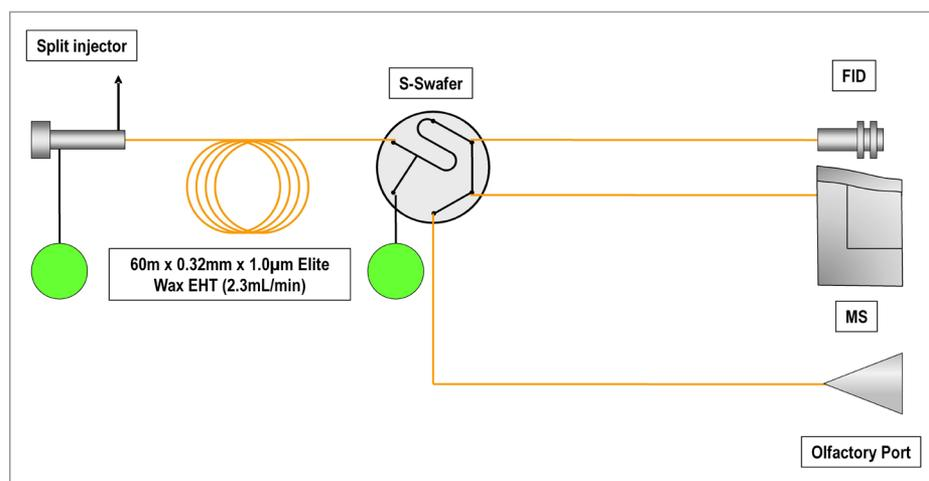
Figure 1. Schematic diagram of the GC system.
