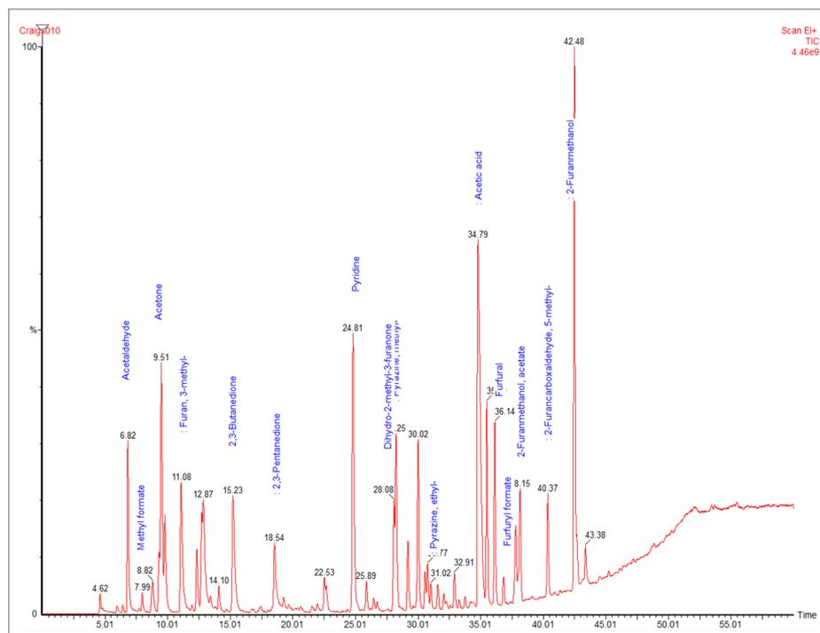
Figure 3. Typical chromatogram from 1 g coffee grains.
