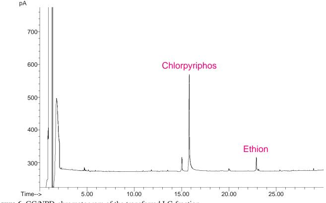
Figure 6. GC/NPD-chromatogram of the transferred LC-fraction.
