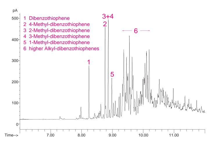
Figure 3. GC/FID-chromatogram of the transferred LC-fraction.
