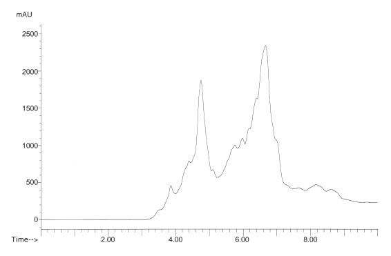
Figure 2. HPLC chromatogram of a crude oil sample.
