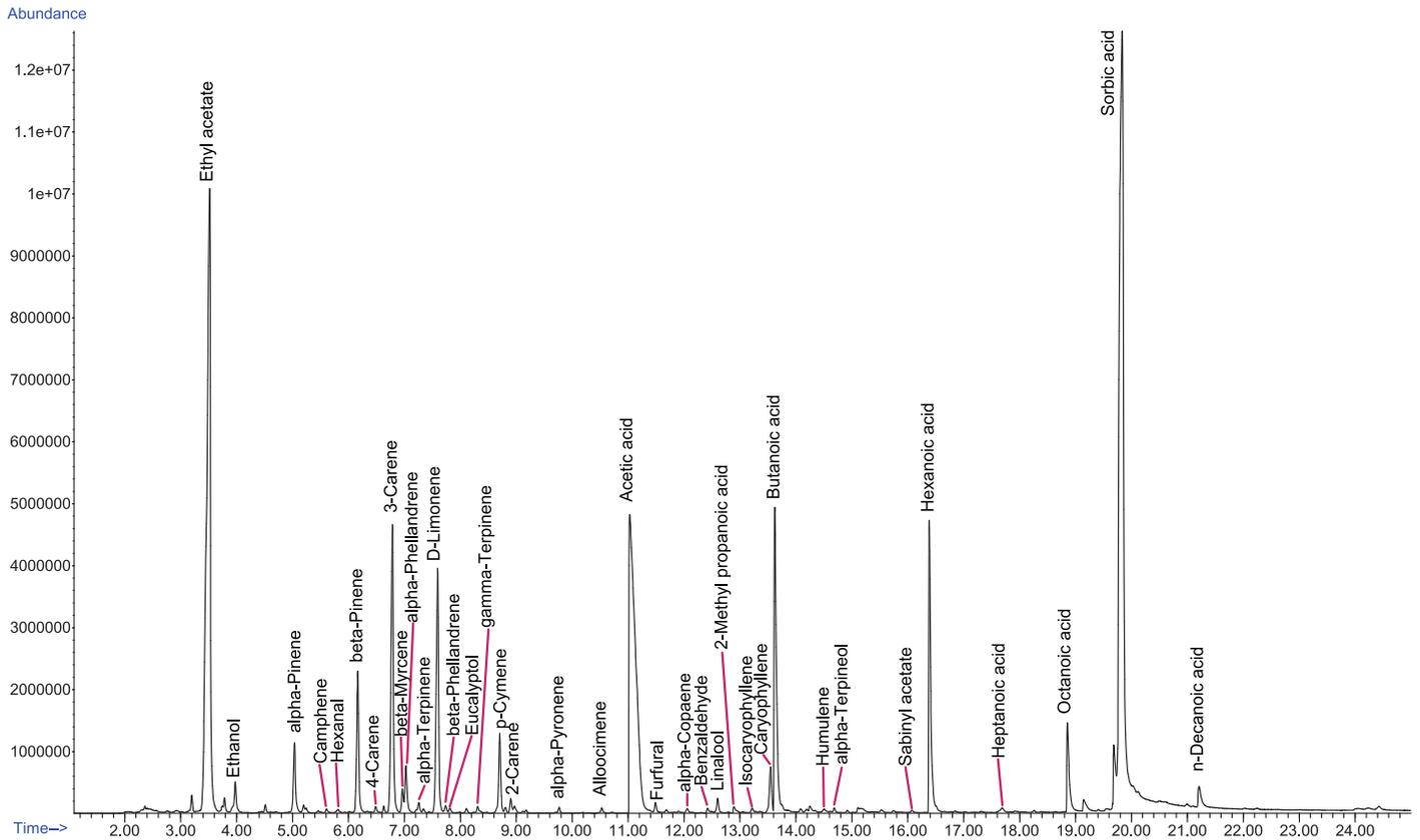
Figure 3. Total Ion Chromatogram resulting from Thin Film Solid Phase Microextraction of Blue Cheese.
