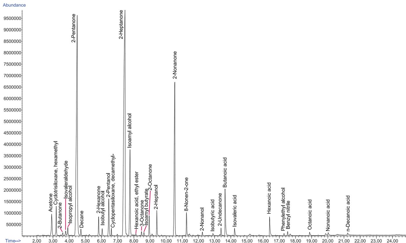
Figure 2. Total Ion Chromatogram resulting from Thin Film Solid Phase Microextraction of Blue Cheese.
