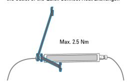
4 Position the heat exchanger in the groove of the MCT heater block and prepare column holders to fix the heat exchanger.
