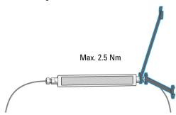
**3** Connect the column connection capillary 0.075 mm x 105 mm to the outlet of the Quick Connect Heat Exchanger.
