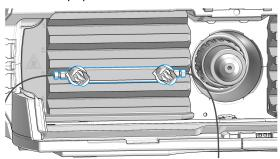
5 Turn column holders to fix the Quick Connect Heat Exchanger in the MCT.
