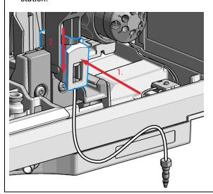
6 Reconnect the seat capillary to the injection valve.
