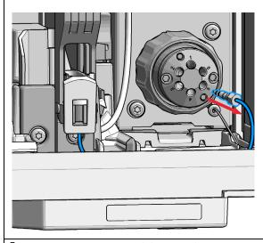
4 Slightly pull (1.) the front clip which holds the needle seat in position. Then carefully lift up (2.) the complete leak tube needle assembly from the holder.
