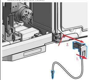
5 Insert the new Needle seat (1.). Press it firmly in position (2.).
