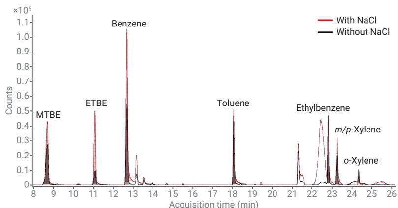
**Figure 2.** Chromatogram of 0.8 ppb BTEX standard analyzed by a 120 µm CAR WR/PDMS SPME Arrow with NaCl (red trace) and without NaCl (black trace).
