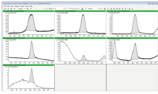
Figure 7. An 120 µm CAR WR/PDMS Arrow MDL replication (BTEX targets shown).
