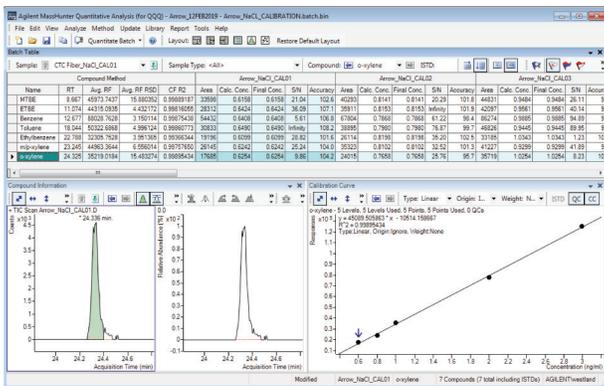
Figure 5. Agilent MassHunter Quant Batch view of 120 µm CAR WR/PDMS Arrow calibration (o-xylene shown).
