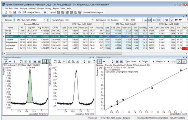
Figure 4. MassHunter Quant Batch view of 85 µm CAR WR/PDMS Fiber calibration (benzene shown).
