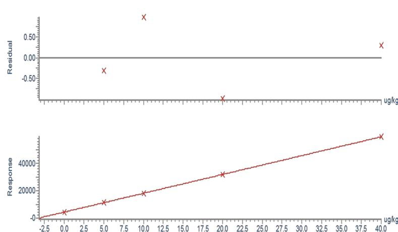
Figure 6: Standard addition plot for the quantification of incurred perchlorate residue in infant food, calculated at a concentration of 0.003 mg/kg (1.5ng/ml in vial).
