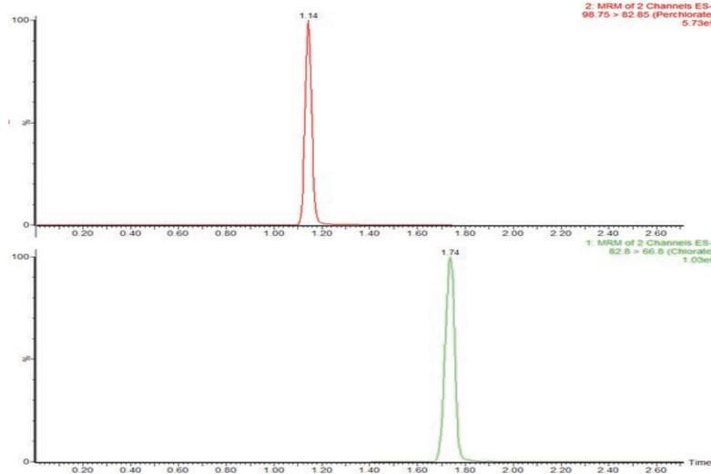
Figure 2: Example of retention and separation of chlorate and perchlorate in infant food (0.010mg/kg) on the TORUS DEA column using the ammonium formate gradient.
