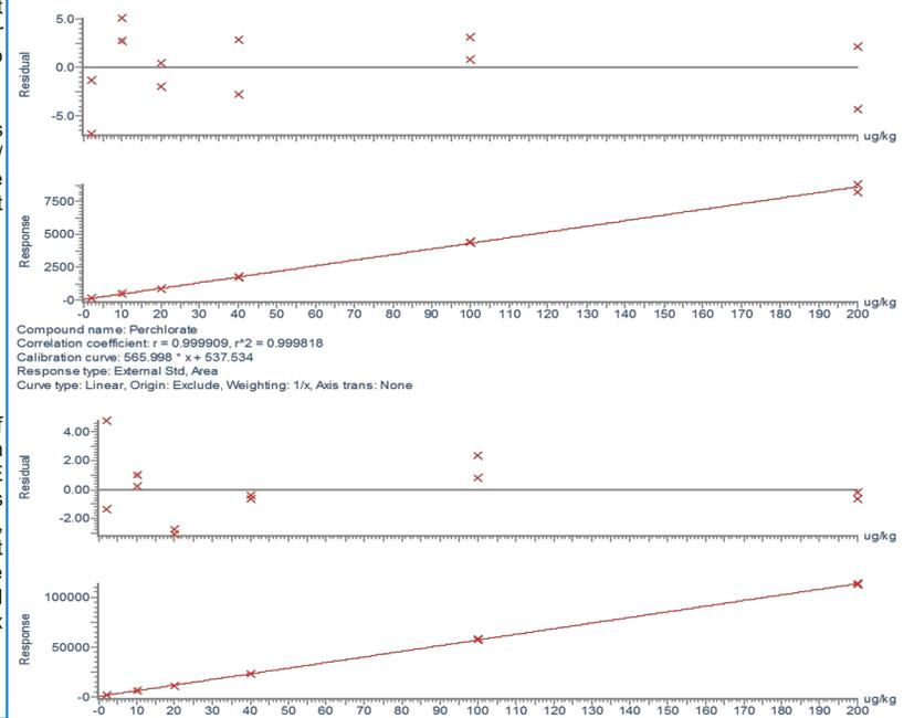
Figure 3: Bracketed matrix matched calibration curve in organic carrot, 0.002mg/kg - 0.2mg/kg (1.0 - 100 ng/ml in vial)
