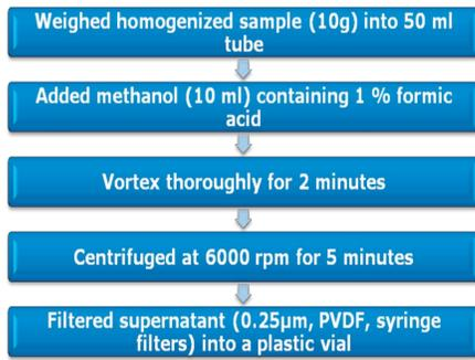
Samples of various food commodities were extracted using the QuPPE method as shown in Figure 1. Filtered extracts were then analysed using the liquid chromatography, mass spectrometry method highlighted below.
