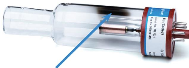
**Characteristic black “getter” patch from unique lamp processing. May also see some cathode material deposited during lamp processing**
