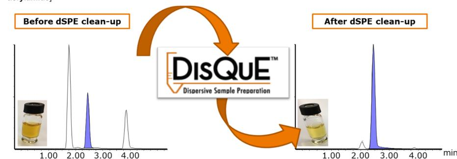
**Figure 1.** Example of extracts and chromatography achieved for ground coffee beans, following QuEChERS extraction without any cleanup and with dSPE cleanup, respectively. Applying cleanup **removes matrix complexity**, yielding cleaner extracts and more selective chromatography. The integrated peak show acrylamide.
