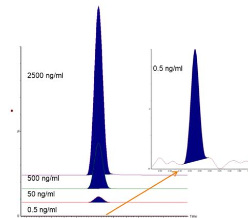
**Figure 3.** Example of quantifier ions achieved for the calibration range in Figure 2, thus showing excellent sensitivity and linearity (without saturation) over an extended concentration range.
