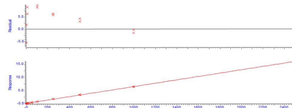
**Figure 2.** Calibration graph for acrylamide prepared in water (internal standard corrected) over the range of 0.5 to 2500 ng/ml with a linear fit and 1/x weighting, yielding  $r^2 = 0.999$ . All back calculated (residuals) concentrations are within 20%.
