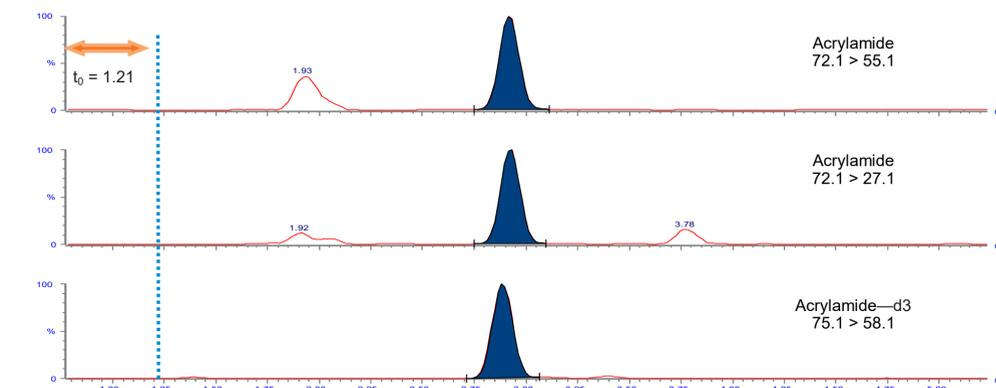
**Figure 4.** Chromatogram of an extracted, FAPAS coffee reference sample, measured at 244 µg/kg. The  $t_0$  of the column ran at the 0.2 mL/min flow rate is indicated on the chromatogram, highlighting the **excellent retention** achieved with a simple LC gradient.
