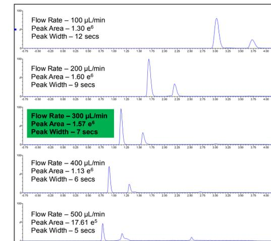
Figure 4) Representative chromatograms showing effect of flow rate for Fluticasone Propionate
