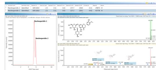
Figure 6. Negative ion HDMS<sup>E</sup> precursor/product ion spectra for neohesperidin food additive, where two mobility separated species have been observed (<sup>13</sup>C<sub>13</sub>CCSN<sub>2</sub> = 228.2 and 238 Å<sup>2</sup>).
