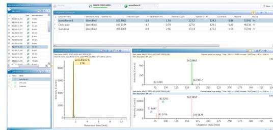
Figure 3. Negative ion HDMS<sup>E</sup> precursor/product ion spectra for acesulfame K detected in a colourless tonic drink (D 4). Additives E 330, E 955 and E969 identified.
