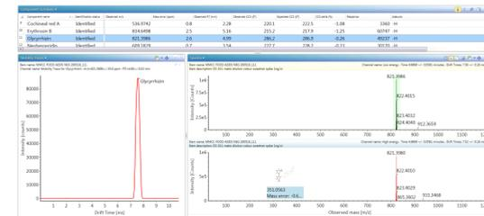
Figure 5. Negative ion HDMS<sup>E</sup> precursor and ion mobility product ion spectra for illegal glycyrrhizin food additive spiked into a colourless tonic drink (D 4). Observed <sup>13</sup>C<sub>13</sub>CCSN<sub>2</sub>=286.2Å<sup>2</sup> (CCS delta= -0.26%).
