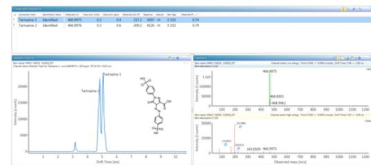
Figure 7. Negative ion HDMS<sup>E</sup> precursor and ion mobility product ion spectra for food additive library constituent tartrazine, where two mobility separated species have been observed (<sup>13</sup>C<sub>13</sub>CCSN<sub>2</sub> = 209.2 and 217.2 Å<sup>2</sup>).
