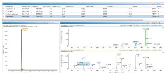
Figure 2. Negative ion HDMS<sup>E</sup> precursor/product ion spectra for aspartame detected in a strawberry and kiwi soft drink (D 3). Colouring and sweeteners identified.
