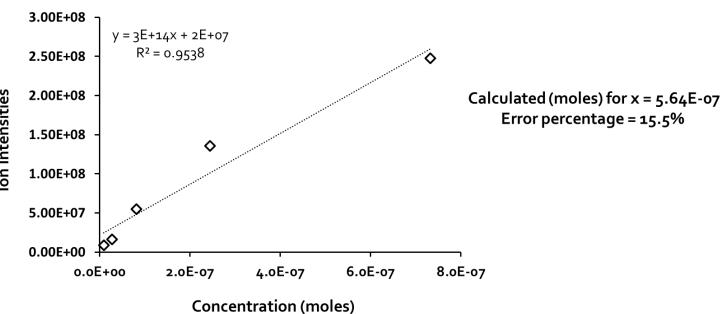
*Figure 5.* The peak intensity of ROI corresponding each concentration was exported as an individual mass spectrum. The ion intestines of analyte standard for each plot was plotted and fitted with linear trendline. Based on the equation, unknown concentration for X was calculated. The error was calculated based on real known concentration of the X.
