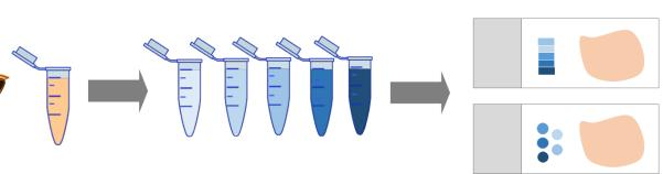
Figure 7. Workflow for future experiments with quantitative DESI imaging using mimetic model of either spiked homogenate spots or section band. This mimetic model ensures a similar degree of analyte extraction and ion suppression as analytes.
