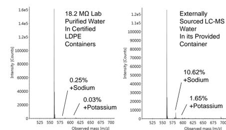
Figure 8. Mass spectra of the 2:T13 peptide as acquired with 0.1% purified DFA modified mobile phases.
