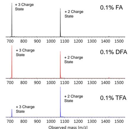
Figure 5. Mass spectra of the 2:T14 peptide from a peptide mapping separation of the mAb Tryptic Digestion Standard using 0.1% FA, purified DFA, or TFA modified mobile phases and an ACQUITY UPLC Peptide BEH C18, 130  $\text{\AA}$ , 1.7  $\mu$ m, 2.1 x 150 mm column.
