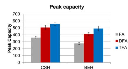
Figure 6. Effective peak capacities based on 8 tryptic digestion peptides.
