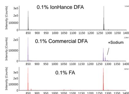
Figure 7. Mass spectra of the 1:T37 peptide from a peptide mapping separation of the mAb Tryptic Digestion Standard using 0.1% purified DFA, commercial DFA, or FA modified mobile phases.
