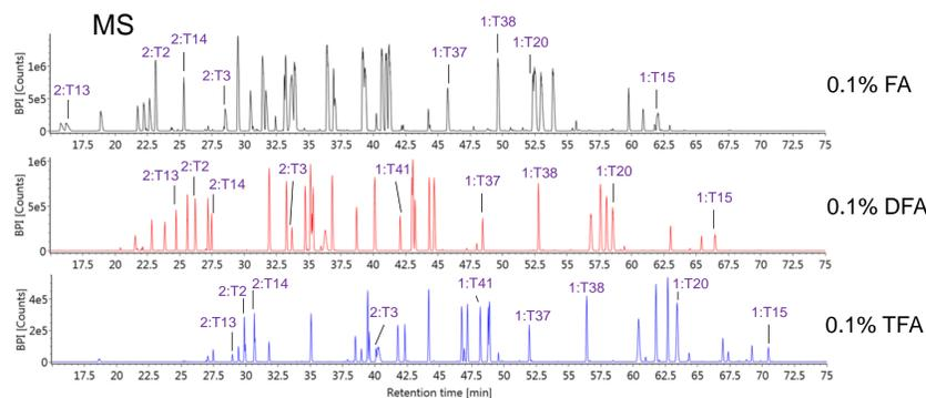
Figure 3. Representative BPI chromatograms from a peptide mapping separation of the mAb Tryptic Digestion Standard using 0.1% FA, purified DFA, or TFA modified mobile phases and an ACQUITY UPLC Peptide BEH C18, 130  $\text{\AA}$ , 1.7  $\mu$ m, 2.1 x 150 mm column.
