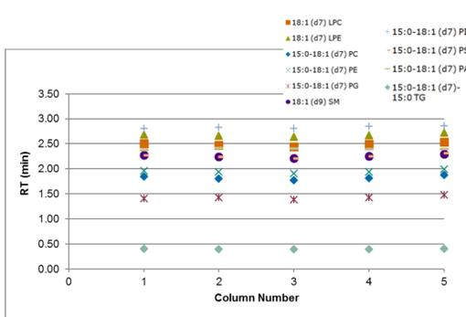
Figure 5. Average retention time (n=1500) of SPLASH LIPIDOMIX™ lipid standard mixture in IPA using five columns from different batches with RSD's <2%.
