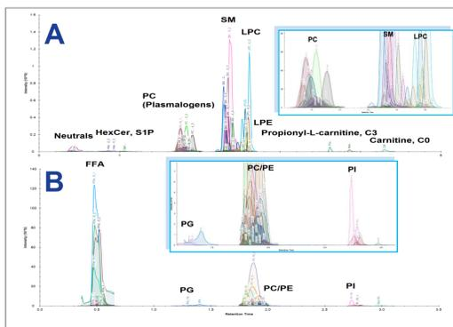
Figure 6. Example chromatogram of plasma samples analysed using Lipid-Quan platform. (A) Positive mode screen (with zoomed insert) and (B) Negative mode screen (with zoomed insert) of various lipid classes.
