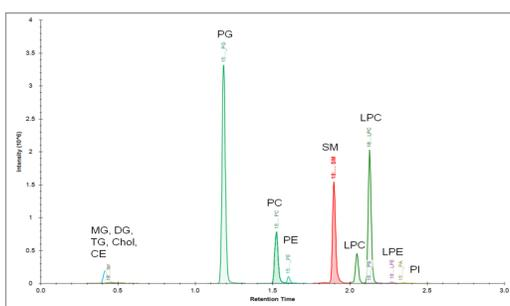
Figure 3. Positive ion mode chromatogram representing HILIC separation of the SPLASH LIPIDOMIX™ lipid standard mixture.
