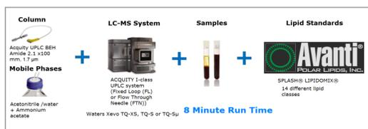
Figure 2. LipidQuan instrumentation and LC-MS/MS conditions. The LipidQuan Quanpedia method file contains LC conditions, MS method with over 2000 MRM transitions and processing methods.
