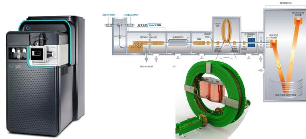
The Waters SELECT SERIES Cyclic Ion Mobility QTOF MS. The cyclic ion mobility module is between the quadrupole and TOF detector. Fragmentation is possible prior to, after, or within the Cyclic IMS module. IMS/IMS & IMS<sup>n</sup> (w/ion selection) are novel supported modes of operation.
