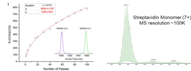
Ion Mobility resolution is scalable by selecting the number of cycles of IMS separation, with IMS resolution ( $\Omega/\Delta\Omega$ ) increasing as the square root of the number of cycles. 100 IMS cycles generates ~800 IMS resolution, with an ion signal loss of only ~1% per cycle. TOF Detection can be acquired with selectable MS resolution of 60,000 (V-Optics) to 100,000 (W-Optics).
