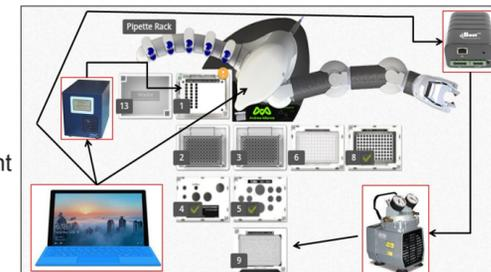
Figure 6: Diagram showing the deck layout of the Andrew system along with the automated control pathways. Features of the control system are outlined in red and include: A) the Surface Pro laptop from Microsoft which runs the Andrew Lab control software to orchestrate B) the INHECO TEC controller for the heating/cooling Domino and C) the iBoot G2+ Advanced Network Power Switch which can switch on/off the vacuum unit which controls suction to the μElution plate Domino.
