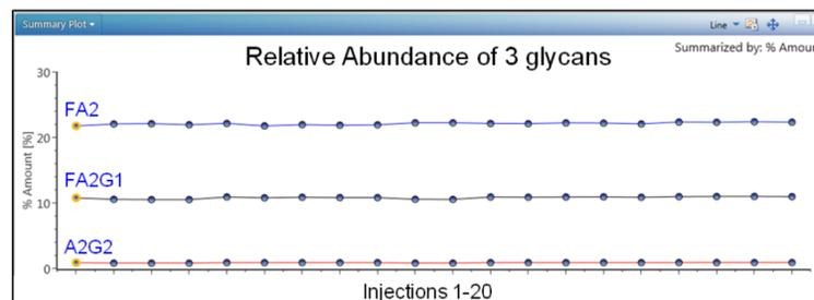
Figure 2: Reproducibility of the LC system demonstrated by monitoring 3 glycoforms of varying relative abundances over 20 consecutive injections. Sample was Waters' RFMS glycan standard. Relative abundance was calculated based on the ratio of area for selected peaks vs the total calculated peak area for all glycoforms.
