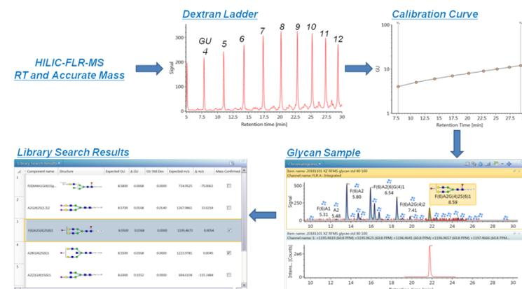
Figure 3: The "Glycan FLR with MS confirmation" workflow within UNIFI. Retention times of glycans are calibrated against a dextran ladder standard, converted to Glucose Unit (GU) values, paired with accurate mass information to conduct a Glycan Scientific Library search within UNIFI for peak identification.
