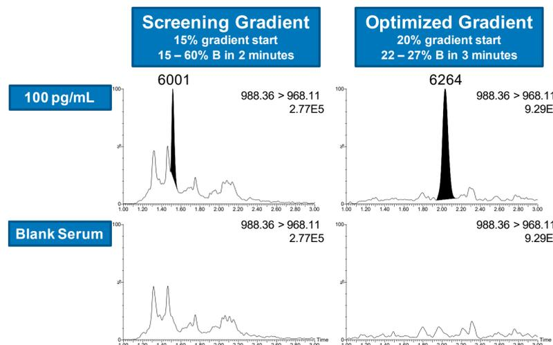
Figure 3. Matrix suppression and chromatographic interferences were significantly decreased by adjusting the chromatographic gradient.
