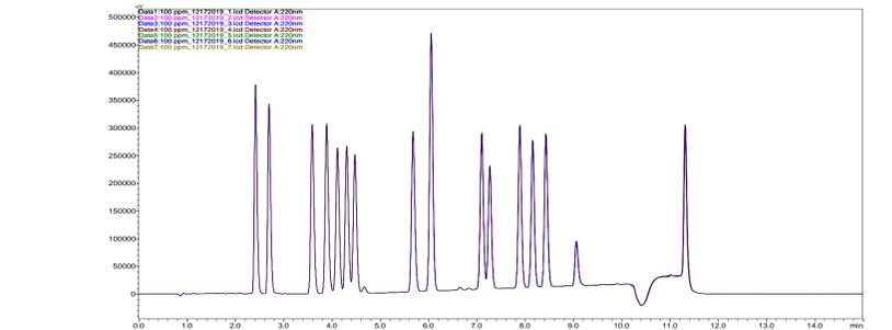
Figure 3: The 15-cannabinoid mixture - Overlay of seven injections (5 µL injection at 100 ppm)
