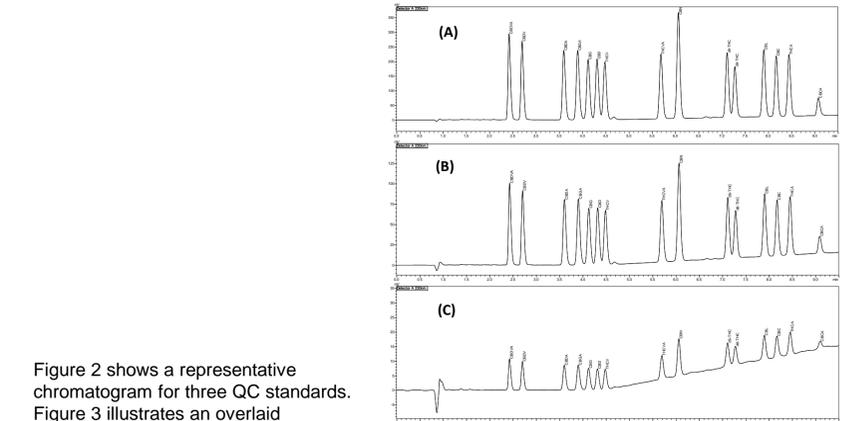
Figure 2: A representative chromatogram showing quality control standards. A 5 µL of (A) QC high, (B) QC medium and (C) QC low
