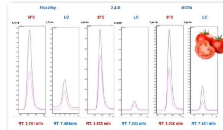
Figure 3: Examples of some compounds that increase their sensitivity using SFC-MS/MS.100 µg/kg tomato
