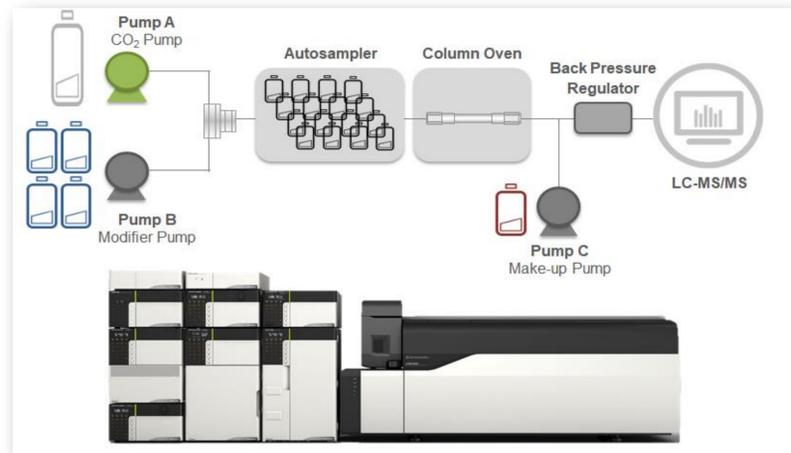
Figure 1: Shimadzu SFC-MS/MS system Nexera UC
