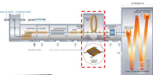
**Figure 1. SELECT SERIES™ Cyclic IMS QToF Mass spectrometer.**
