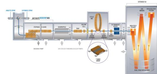
**Figure 1.** Schematic of Cyclic IMS, with the cIM device embedded in a Q-cIM-ToF geometry.
