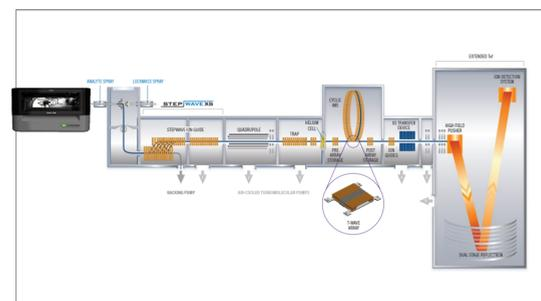
Figure 1. The Select Series Cyclic IMS mass spectrometer geometry is illustrated here.
