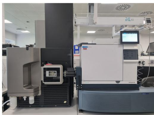
Figure 1. GC coupled to the APGC and Xevo G3 QToF mass spectrometer.
