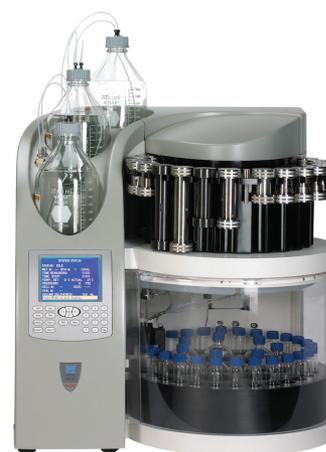
Figure 2. ASE 350 Accelerated Solvent Extractor
