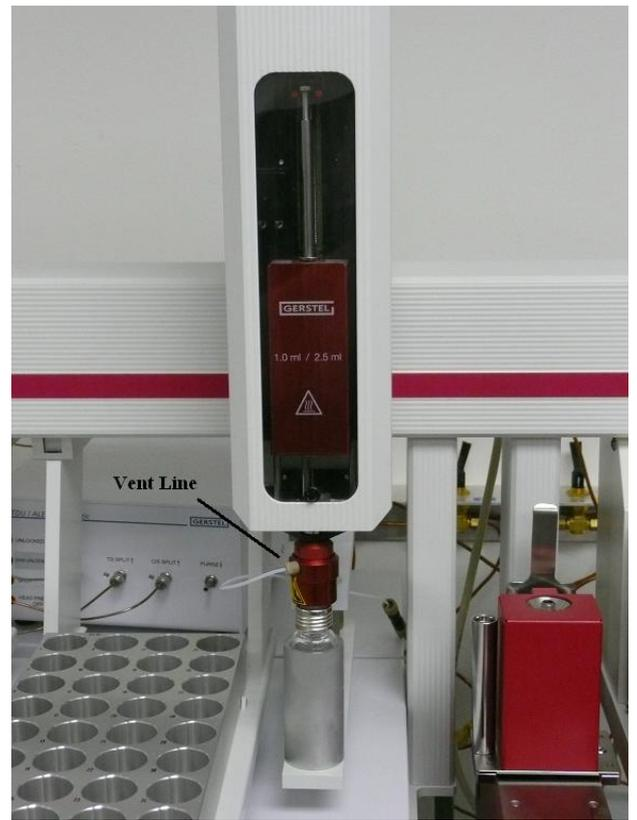
**Figure 2.** A vial is being purged in the MPS.
