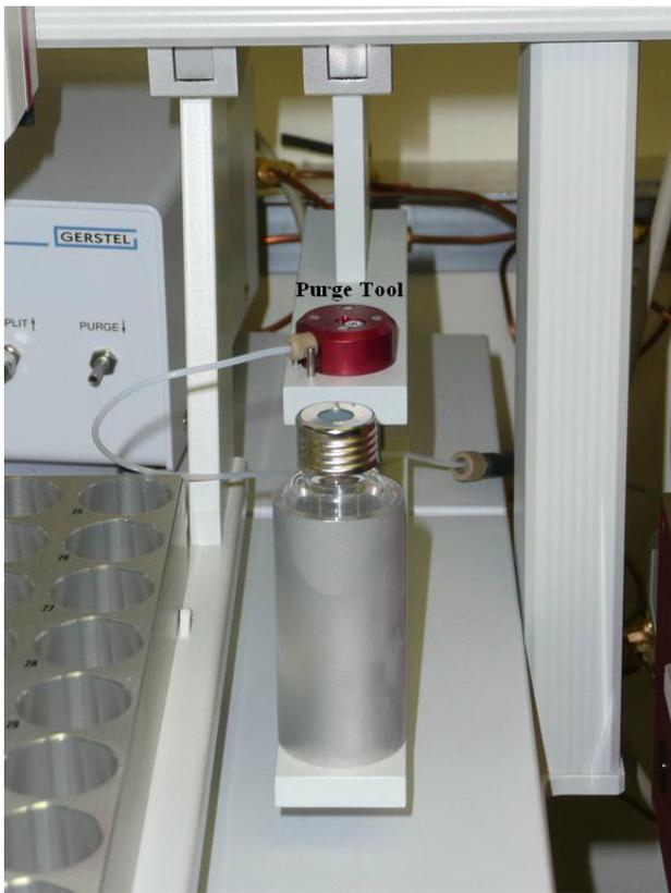
**Figure 1.** Purge tool and purge tool holder.
