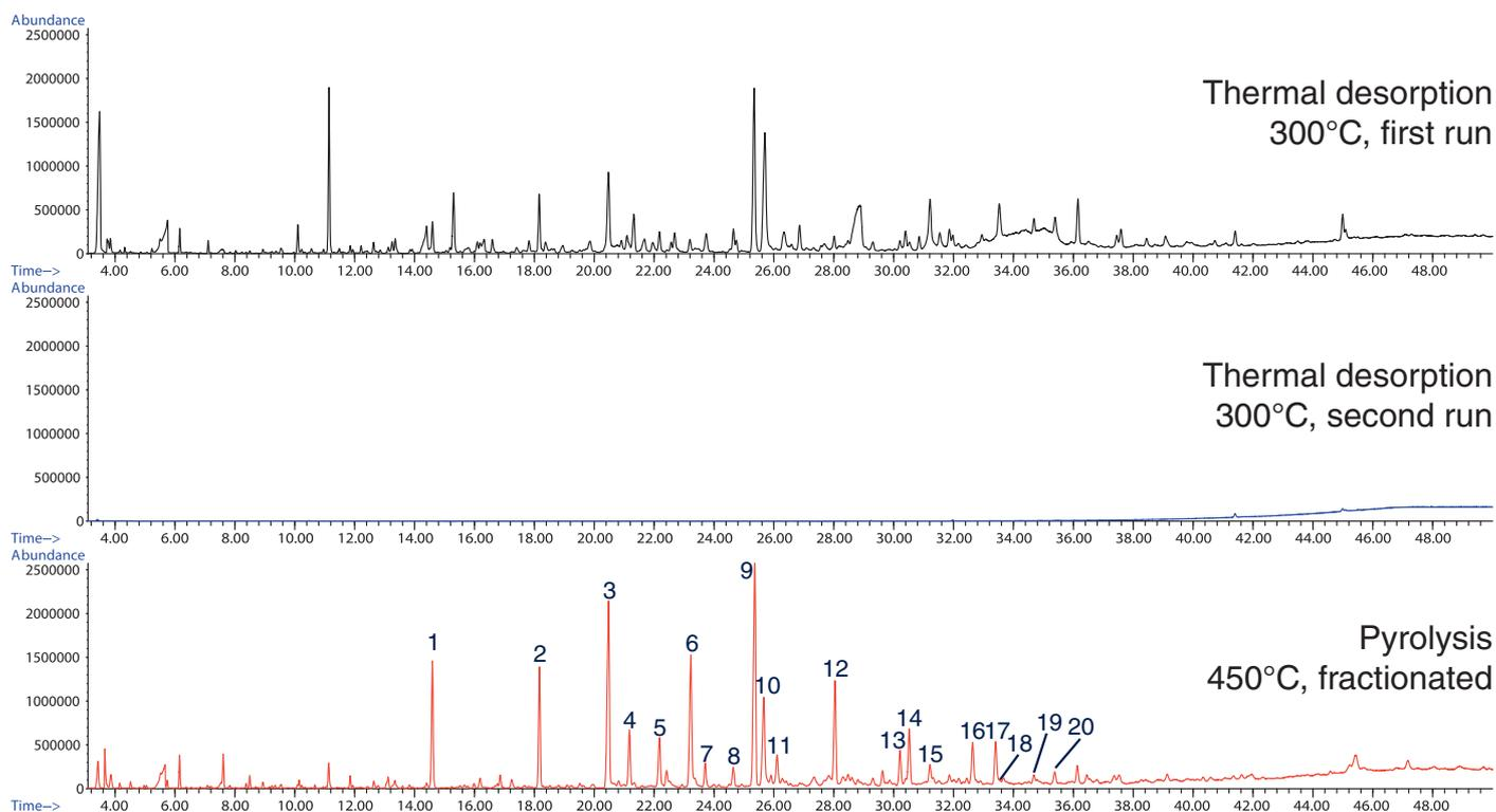
**Figure 2.** Comparison of TICs resulting from the first and second thermal desorption of QR whiskey residue at 300°C and from fractionated pyrolysis of the same sample at 450°C directly after the thermal desorption steps.
