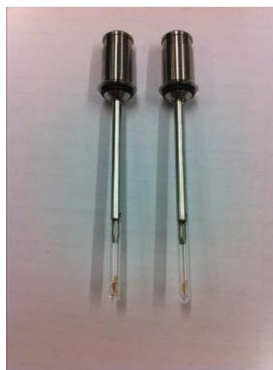
**Figure 1b.** QA and QR wood chips in pyrolysis sample holders.
