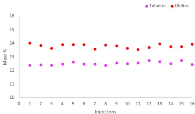
**Fig 5.** Repeatability data of Toluene and Olefins
