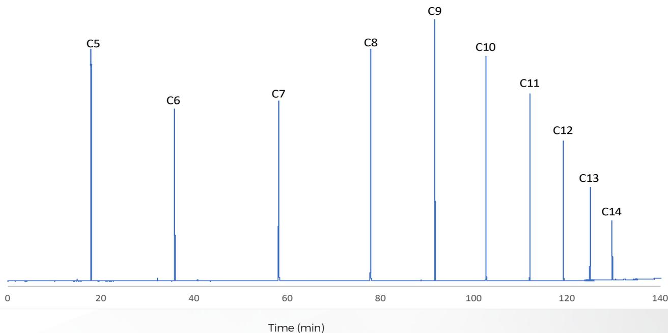
**Fig 1.** C<sub>5</sub>-C<sub>14</sub> n-paraffin calibration standard Time (mins)
