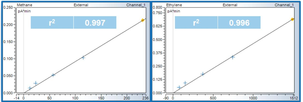
Figure 4. Low-level calibration curves for methane and ethylene.
