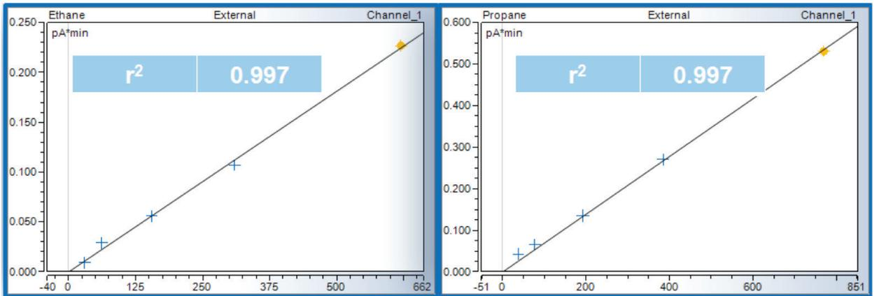
Figure 5. Low-level calibration curves for ethane and propane.
