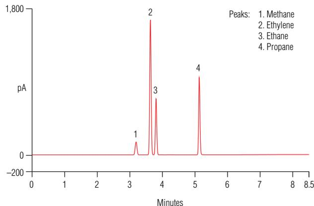
Figure 2. Chromatogram of the four gases analyzed (highest calibration point). In order from left to right, the peaks represent methane, ethylene, ethane, and propane.
