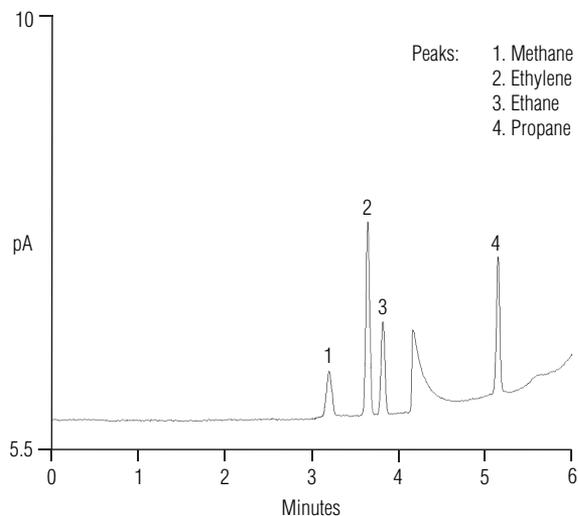
Figure 3. Chromatogram of the four gases analyzed (second calibration point, 10 µL added).
