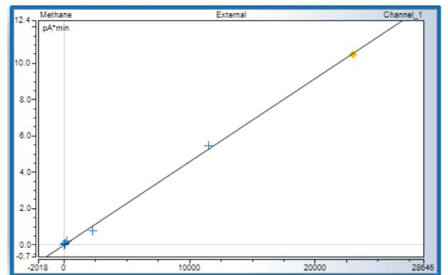
Figure 6. High-level calibration curve for methane.
